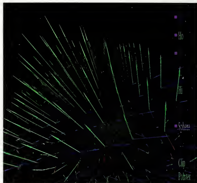
Figure 2. Image of the electric, magnetic, and energy field vectors in a single time step in the simulation of resonant optical scattering by metamagnetic materials.
